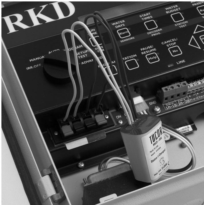
Figure 4.12. How to connect a decoder to the controller
