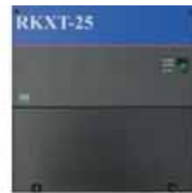
An RKS with WIN-100 RealNet cellular connection, configured as a "Group" node. The RKS wirelessly controls three RKXT-25 extensions, controlling 1 - 100 valves.
